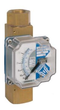
The AMD limit switch consists of a NAMUR slot type inductive sensor, that is actuated by a vane. Given that there is no physical contact in the operation, the limit switch has no influence on the indicator needle movement. A NAMUR amplifier with a relay output can be supplied as an optional element
